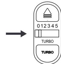
4. The mixer starts mixing immediately. To avoid splashing, we recommend always starting at the lowest level (level 1) and increasing the speed as required by sliding the switch during use.
